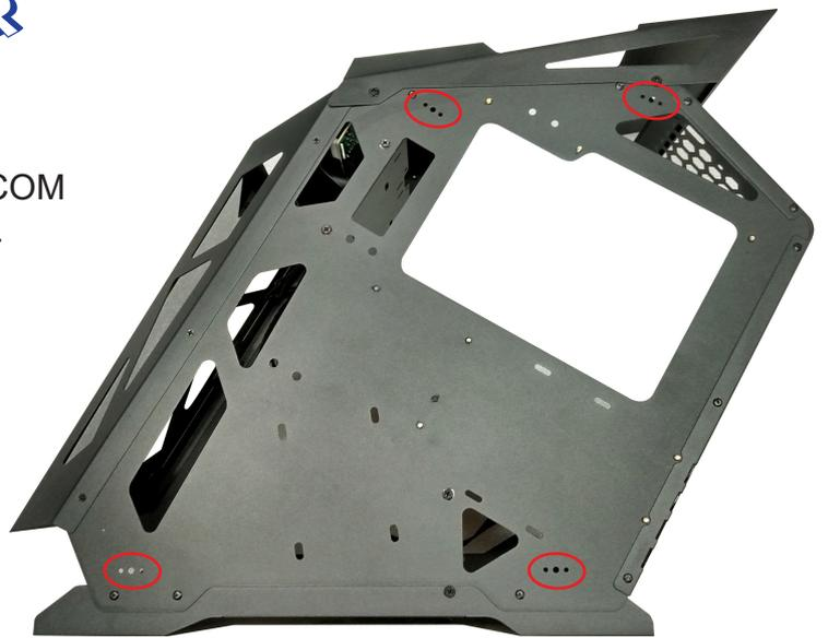
2- COM UMA CHAVE PHILIPS, PARAFUSE OS SUPORTES COM O PARAFUSO INTERNO.
